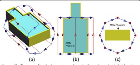
Figure 4 The illustration of the simulation setup to determine the maximum electric field location inside the ASTM phantom.
