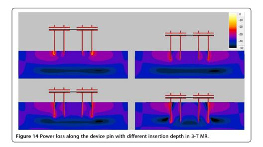
induced current on the bar which results in less power loss in the pin, and thus lower temperature rise.
