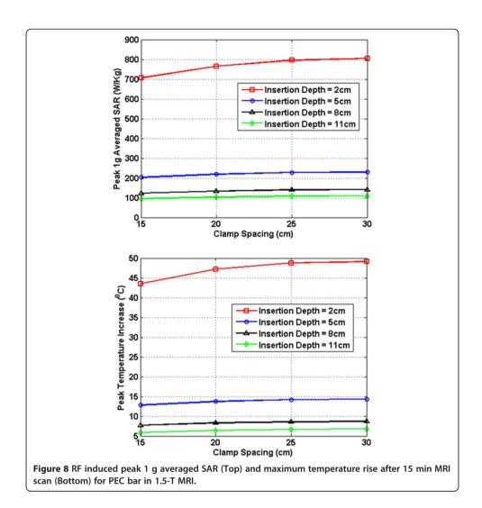
Electromagentic simulations are first conducted to determine electromagnetic energy deposition near the pins of the devices. Then, thermal simulations are carried out to estimate the temperature rise near the tips. Based on the energy deposition near the device tips, the temperature rise in ASTM phantom is calculated using the heat transfer equation given as:
