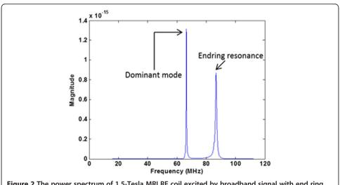
Figure 2 The power spectrum of 1.5-Tesla MRI RF coil excited by broadband signal with end ring tuning capacitance = 7.2 pF.
