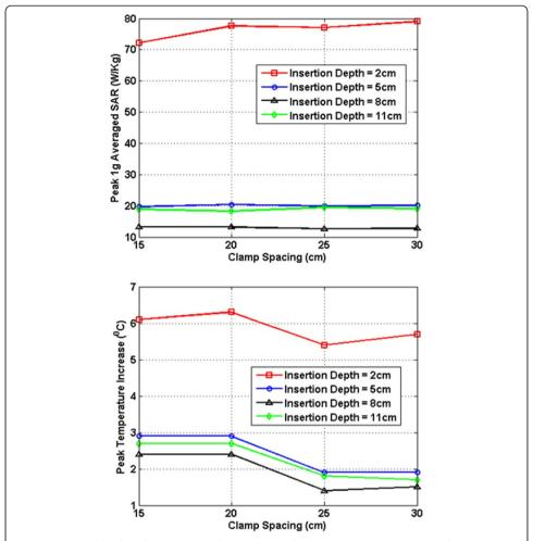
**Figure 12** RF induced peak 1 g averaged SAR (Top) and maximum temperature rise after 15 min MRI scan (Bottom) for plastic glass bar in 3-T MRI.
