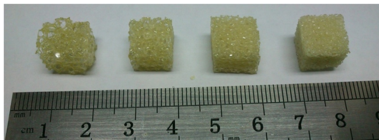
Figure 1 The cellular synthetic bone used in this study [from left (Group 1) to right (Group 4): 0.12 \text{ g/cm}^3 , 0.16 \text{ g/cm}^3 , 0.20 \text{ g/cm}^3 , and 0.32 \text{ g/cm}^3 ].
