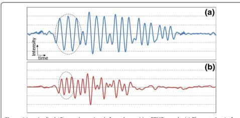
**Figure 4** Longitudinal 1D transducer signals from the positive PTMF sample: (a) Elements 2 – 6 of Group 0; (b) Elements 1 – 6 of Group 1. The scales of x-axes of (a) and (b) are identical. Dashed circles indicate the signal from the largest element of each group.
