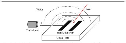
**Figure 1 Illustration of the sound propagation in water.** Ultrasound generated at the chromium strips propagates along the surface of the fused silica plate in the form of shear wave (solid arrow) and in the form of bulk wave (dashed arrow).
