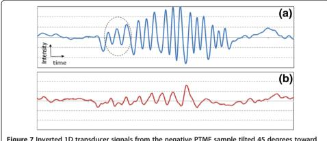
**Figure 7** Inverted 1D transducer signals from the negative PTMF sample tilted 45 degrees toward the transducer: (a) Elements 2 – 6 of Group 0; (b) Elements 1 – 6 of Group 1. The scales of x-axes of (a) and (b) are identical. Dashed circles indicate the signal from the largest element of each group.
