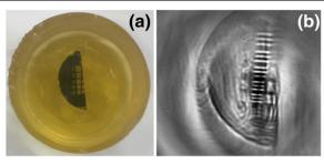
Figure 8 (a) Digital photography of the suggested resolution target. A piece of PTMF sample with only Group 0 patterns was embedded in a gelatinous block; (b) 2D reconstruction of PAT image from the suggested resolution target. Inverted signal was used for this particular resolution target made of negative PTMF sample.
