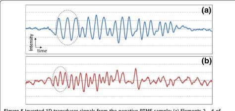
**Figure 5** Inverted 1D transducer signals from the negative PTMF sample: (a) Elements 2 – 6 of Group 0; (b) Elements 1 – 6 of Group 1. The scales of x-axes of (a) and (b) are identical. Dashed circles indicate the signal from the largest elements of each group.
