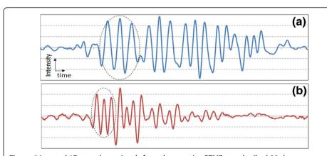
**Figure 6** Inverted 1D transducer signals from the negative PTMF sample tilted 30 degrees toward the transducer: (a) Elements 2 – 6 of Group 0; (b) Elements 1 – 6 of Group 1. The scales of x-axes of (a) and (b) are identical. Dashed circles indicate the signal from the largest elements of each group.
