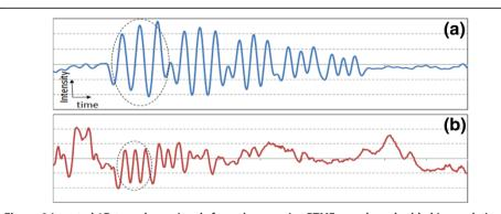
Figure 9 Inverted 1D transducer signals from the negative PTMF sample embedded in a gelatinous block. (a) Elements 2-6 of Group 0; (b) Elements 1-6 of Group 1. The scales of x-axes of (a) and (b) are identical. Dashed circles indicate the signal from the largest element of each group.
