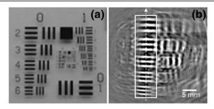
**Figure 3** (a) Digital photography and (b) a full 360 degree PAT image of the positive PTMF sample. Patterns within the white rectangle represent Elements 2–6 of Group 0. Dashed-arrow represents the direction of 1D intensity profile measured by the transducer at a single fixed position.
