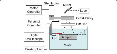
**Figure 2 Schematic of the PAT setup.** Solid black lines represent electrical connections, dashed lines represent laser paths, and red line represents ultrasound path. TR is the transducer. PTMF sample is placed such that the metal film is facing toward the incoming laser.
