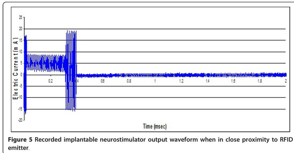
pulse of 134 kHz) sine-wave pulse is approximately 40 mA [[18], Figure 4.16]. The RFID pulse of 134 kHz in frequency is significantly higher in frequency than pulses generated by spinal cord neurostimulator system and therefore must be much higher in amplitude in order to generate an action potential.
