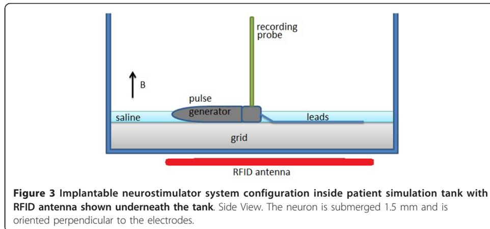
The neurostimulator system was configured so that the leads outline the RFID antenna and the extra length was looped around the outline of the corners of the antenna (Figure 2). The magnetic field around the corners of the antenna was previously recorded to generate the highest magnetic field strengths. This layout represents the worst case scenario for coupling electromagnetic fields into implantable leads. The worst case scenario layout was also verified experimentally.
