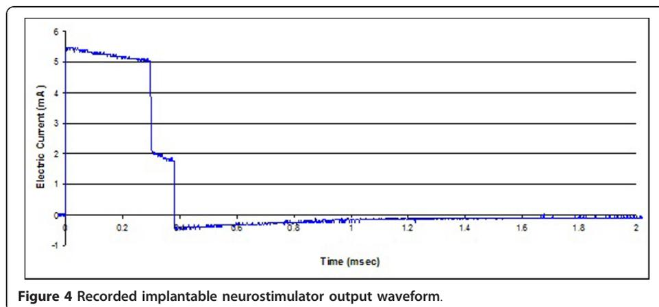
**Figure 4** Recorded implantable neurostimulator output waveform.
