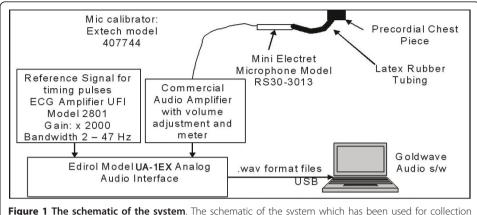
**Figure 1 The schematic of the system**. The schematic of the system which has been used for collection of the preliminary data.
