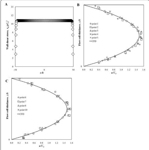
Figure 5 Streamwise velocity profile of flow in the parallel-plate flow chamber determined using micro-PIV and CFD. Streamwise velocity characterization (A) along the center and (B) in proximity of the side walls. (C) Shear stress distribution along the channel span at z/h = 0, 1. (B) A peak at coordinates  $(x, y) = (250 \ \mu\text{m}, 650 \ \mu\text{m})$  and (C) a trough at coordinates  $(x, y) = (300 \ \mu\text{m}, 350 \ \mu\text{m})$ .
