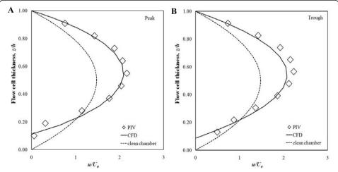
Figure 6 Local distortion of the streamwise velocity profile due to endothelial cell topography. Velocity profiles were determined at point 6 from Figure 1B; (A) peak  $(x, y) = (250 \ \mu\text{m}, 650 \ \mu\text{m})$ ; (B) trough  $(x, y) = (300 \ \mu\text{m}, 350 \ \mu\text{m})$ .
