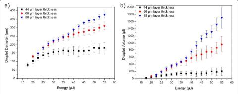
Figure 6 Comparison of printed droplet diameter with droplet volume. Progressions of the droplet diameter (a) and the droplet volume (b) depending on layer thickness and laser energy of a solution with  $\eta=0.4311$  Pa·s.
