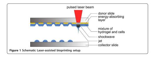
cleaned with acetone before usage. The bottom side of the donor glass slide was coated with a 60 nm gold layer using a plasma-enhanced sputter coater (Cressington 208HR, EO Service GmbH, Germany). The hydrogel layer was applied upon the gold layer by a blade coater. A 60 mm achromatic lens focused the laser beam through the donor-glass slide onto the gold layer.
