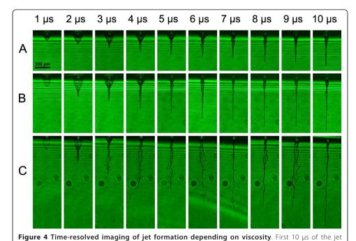
formation depending on the solution's viscosity whereas A corresponds to  $\eta=0.4311$  Pa·s, B to  $\eta=0.1477$  Pa·s and C to  $\eta=0.0218$  Pa·s. Black spherical disturbances in the background of C are due to condensed humidity on the microscope objective.
