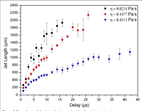
**Figure 3 Dependence of the jet evolution on viscosity**. Plot of the jet length dependence on the temporal delay. Five images per delay have been taken. The error bars mark the standard deviation.
