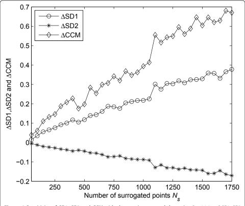
**Figure 4 Sensitivity of SD1, SD2 and CCM with changes in temporal dynamics**. Sensitivity of SD1, SD2 and CCM with number of shuffled points  $N_s$ . At each step the number of shuffled points increased by 50. Each time the signal has been shuffled for 30 times and its mean has been taken to calculated the sensitivity.
