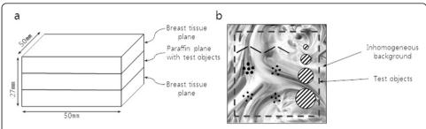
**Figure 5** The breast-mimicking phantom used for the experimental scans. (a) The phantom consists of three layers. The top and bottom layers are simulating inhomogeneous breast tissues. (b) The middle layer having high-intensity feature patterns against the homogeneous background.
