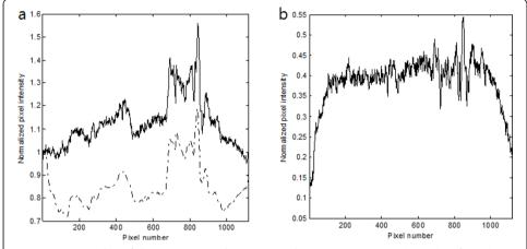
**Figure 10 Examples of the experimental projection data**. (a) A projection data taken from the rat imaging. The solid line represents the measured tomosynthesis projection data and the dashed line represents the projection data computed from the CT images. The computed projection data has been obtained from outside the rectangular ROI shown in Fig. 9b. (b) The subtracted projection data which stems from the ROI.
