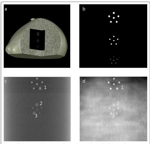
**Figure 4** The breast-mimicking phantom for simulation and its simulated tomosynthesis images. (a) The 3D breast-mimicking phantom for the simulation. (b) The high intensity feature patterns located in the middle of the 3D breast-mimicking phantom. (c) The simulated local tomosynthesis image obtained with the proposed method. (d) The simulated conventional tomosynthesis image. The numbers are the places where CNRs are to be evaluated.
