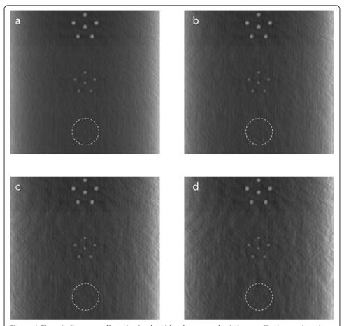
**Figure 6** The misalignment effects in simulated local tomosynthesis images. The images have been obtained with misregistration between the CT and tomosynthesis scan geometry. The misregistrations are made by shifting the CT projection data in the horizontal direction by multiple pixel widths. (a) 0-pixel shift. (b) 2-pixel shift. (c) 4-pixel shift. (d) 8-pixel-shift.
