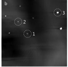
**Figure 8** The experimental tomosynthesis images of the phantom. (a) The image obtained by the proposed method. (b) The image obtained by the conventional method. The numbers are the places where CNRs are to be evaluated.
