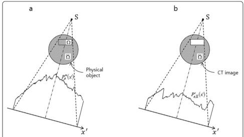
**Figure 2** The two projection data for image reconstruction. (a) The projection data acquired from the tomosynthesis scan. (b) The projection data calculated from the CT image which stems from outside the region of interest.
