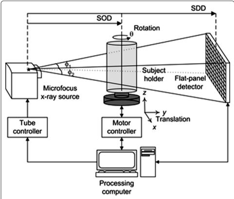
**Figure 3** The micro-CT system used for the CT and tomosynthesis scans. The magnification of the projection image on the flat-panel detector is controlled by changing the source to object distance (SOD).
