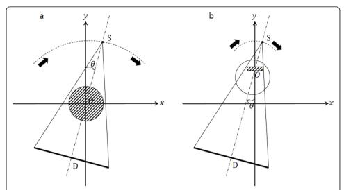
**Figure 1 Scan geometries of the CT and the tomosynthesis.** (a) The CT scan geometry with small magnification. (b) The tomosynthesis scan geometry with big magnification. *S* and *D* represent the x-ray source and detector, respectively, and *O* represents the center of rotation of the scan.
