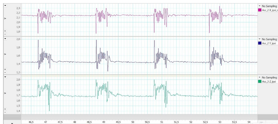
Fig. 10 Illustration of the individual vectors ( x , y , and z axes) of the accelerometer. Three measurements were always averaged for statistical evaluation
