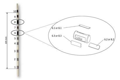
**Fig. 1** Multipolar esophageal catheter equipped with ten electrode sections. All sections contain omnidirectional electrodes, except sections 6 and 8, which include three directed electrodes in the circumference
