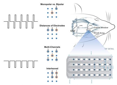
**Fig. 7** Experimental paradigms. The optical window was opened over the primary motor cortex. Electrical stimulation was delivered through an ECoG array. In conditions of monopolar vs. bipolar stimulation and electrode spacing, charge-balanced biphasic square pulses were applied with cathodic (negative) phase first. In conditions of multi-channel configurations and interleaved stimulation, cathodic pulses were applied
