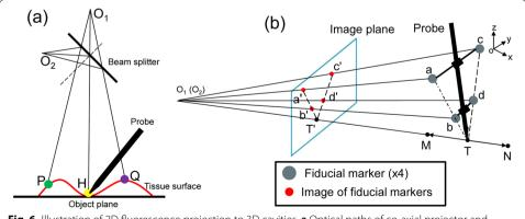
**Fig. 6** Illustration of 2D fluorescence projection to 3D cavities. **a** Optical paths of co-axial projector and camera system. **b** Probe tip detection by fiducial marker tracking, and point-by-point in situ projection
