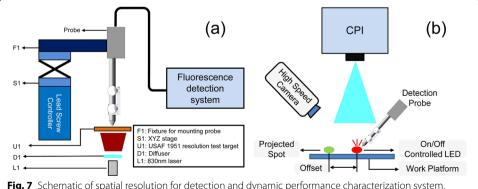
**Fig. 7** Schematic of spatial resolution for detection and dynamic performance characterization system. **a** Schematic of spatial resolution measurement system. **b** Schematic of FSP dynamic performance characterization system
