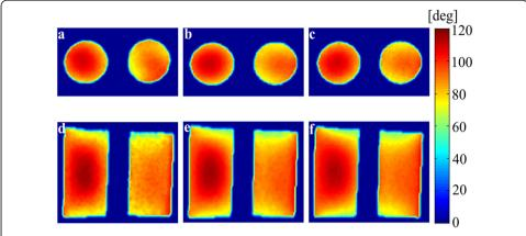
**Figure 7 Flip angle maps obtained by the double angle method (DAM).** The flip angle calibration for the nominal flip angle of 90 degrees has been done by the quadrature excitation **(a,d)**, the iterative RF pulse calibration **(b,e)** and the conventional B1 shimming **(c,f)** for an axial slice **(a,b,c)** and a coronal slice **(d,e,f)**.
