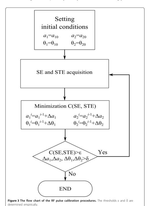
computed from the current echoes  $(SE_j)$  and  $STE_j$ ) and the previous echoes  $(SE_{j-1}, STE_{j-1})$  by minimizing the cost function. Then, the new shimming parameters are used to update the RF pulses to be applied at the next cycle. The acquisition of the echo signals and the computation of the shimming parameters are repeated until either the cost function value becomes smaller than the empirically determined thresholds.
