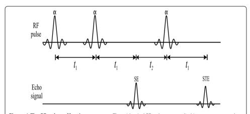
**Figure 1 The RF pulse calibration sequence.** Three identical RF pulses are applied in sequence at each channel of the transmit coil, and the first spin echo (SE) and the stimulated echo (STE) are acquired to determine the magnitudes and phases of the RF pulses to be applied at the next RF pulse sequence.
