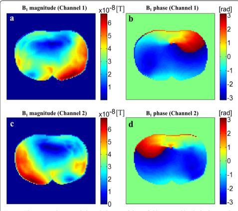
Figure 5 The magnitude (a,c) and phase (b,d) maps of the B1 field generated by the birdcage coil. The top (a,b) and bottom (c,d) rows. The top and bottom rows represent the channel 1 and channel 2 of the birdcage coil, respectively.
