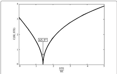
**Figure 2** The cost function value with respect to the ratio of STE to SE. The cost function value becomes 0 radians at the flip angle of 65.5 degrees.
