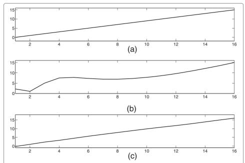
Figure 2 The original signal and its different reconstructed versions. (a) The original signal signal, (b) the reconstructed signal after DFT and IDFT using  $\theta_k = (2k\pi/N)^{0.8}$ , (c) the reconstructed signal after the identical DFT, IDFT and a filtering process using the designed filter between DFT and IDFT.
