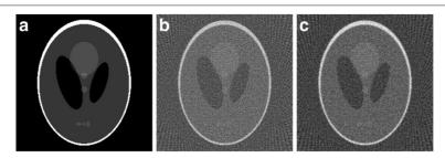
Figure 7 The original image and the reconstructed images using FBP algorithm with different reconstruction filters (N = 256,  $\theta = [0^o, 3^o, \cdots, 177^o]$ ). (a) The original image, (b) using the ramp filter |k/N|, (c) using the designed filter.
