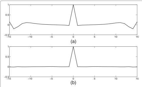
Figure 4 The convolution vectors with and without the reconstruction filter  $(N=16, \theta_k=(2\pi k/N)^{0.8})$ . (a) The convolution vector without the reconstruction filter, (b) with the reconstruction filter designed.
