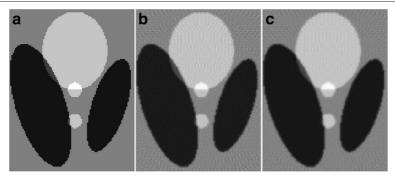
Figure 8 The small regions of original image and the reconstructed images using FBP algorithm with different reconstruction filters (N = 256,  $\theta = [0^o, 1^o, \cdots, 179^o]$ ). (a) The original image, (b) using general filter |k/N| (c) using the designed filter.
