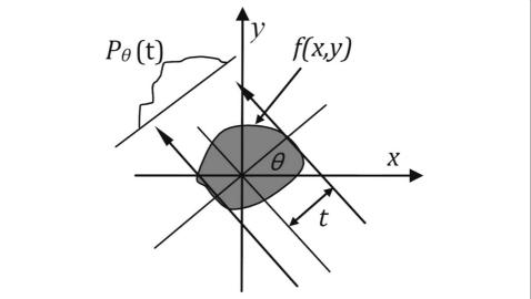
Figure 1 Parallel Projection: an object f(x,y) and its projection  $P_{\theta}(t)$  are shown from the angle  $\theta$ .
