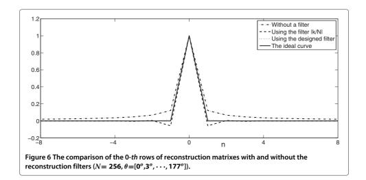
Consider the symmetry of the reconstruction matrix, it implies the designed filter can make  $h_r(n, m)$  be more close to  $\delta(n, m)$  than the ramp filter.
