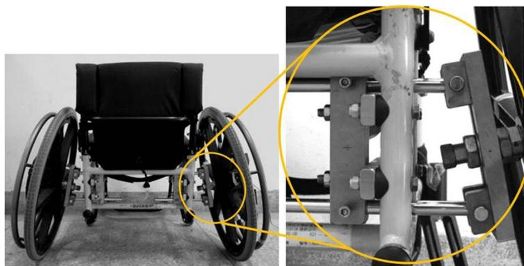
**Figure 1** A self-designed mechanism for rear-wheel camber adjustment. The mechanism was mounted on the wheelchair to adjust the rear-wheel camber.
