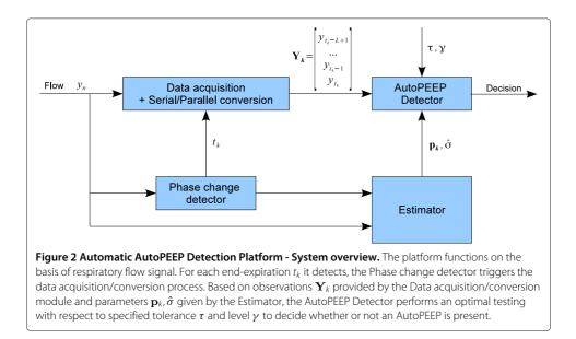
**Data acquisition and Serial/Parallel conversion** This very-first module acquires the discrete flow signal  $y_n$  provided by the ventilator or by an independent flow sensor
