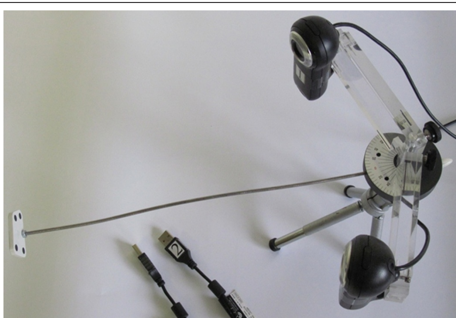
Figure 1 Stereophotogrammetrical tracking device. The plastic fiducial marker (left), consisted of four black circles on a white background, was placed on the pin between the two web cameras.
