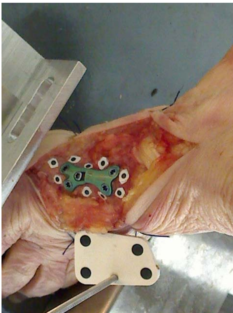
Figure 4 Marker test on the cadaveric foot specimen. The single right camera picture. The nine markers were attached on the first metatarsal bone fragments fixing with a locking screw plate after a proximal osteotomy. The fiducial marker was placed in the middle of the lower image part.
