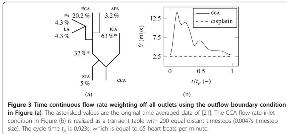
the Fluent™ simulation. In particular a transient table for the CCA and a constant value for cisplatin is used. The volume fraction of the dispersed phase cisplatin was set to 100% at the cisplatin inlet and 0% at the CCA inlet.
