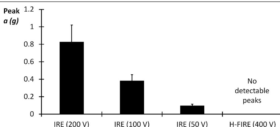
**Figure 6** Peak acceleration ( $a$ ) during IRE protocols averaged over the first 90 pulses. Mean peak acceleration during IRE treatments at the cervicothoracic junction for each applied voltage was significantly different from each other. H-FIRE resulted in no detectable acceleration of the cervicothoracic junction.
