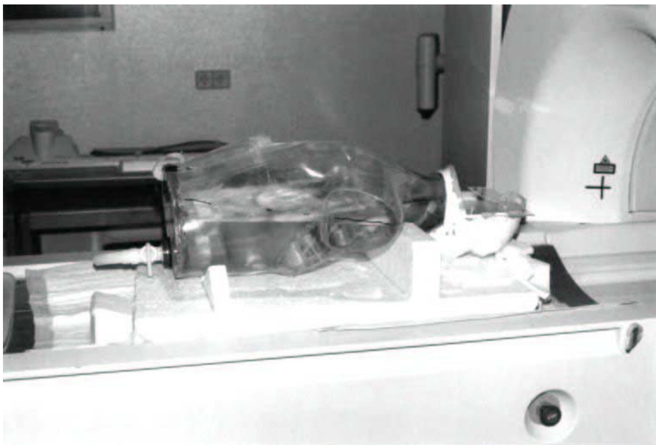
Figure 1 Phantom used in the 1.5 T MRI
