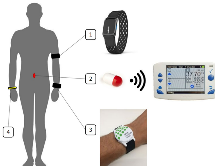
Fig. 5 Schematic representation of the equipment provided to the participants: (1) optical heart-rate monitor on the left upper arm; (2) ingested telemetric pill and readout monitor; (3) wearable CBT sensor on the left wrist; (4) "no-MRI" warning bracelet
