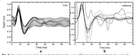
**Fig. 4** Slow time signals at 5.5–6 cm depth obtained by using different detection methods: **a** is using the 7-chip Barker coded detection, and **b** is using traditional pulse-echo detection
