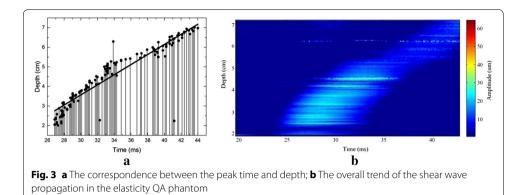
value of the elasticity QA phantom is 2.7–3.1 m/s. The elasticity value measured by our system was within the rational range, which indicated that our system was effective.
