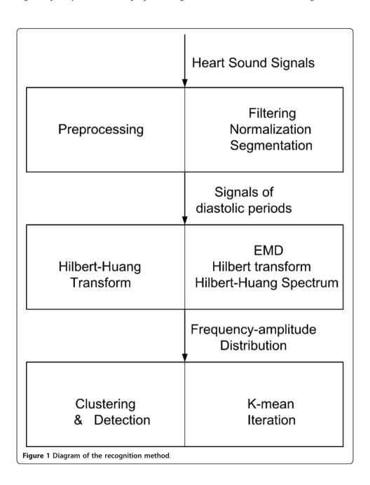
signals were filtered to eliminate the noise, and followed by normalization and segmentation. These steps were illustrated in the following:
