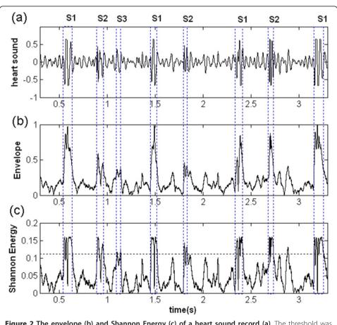
**Figure 2 The envelope (b) and Shannon Energy (c) of a heart sound record (a).** The threshold was shown with a dashed line in (c).
