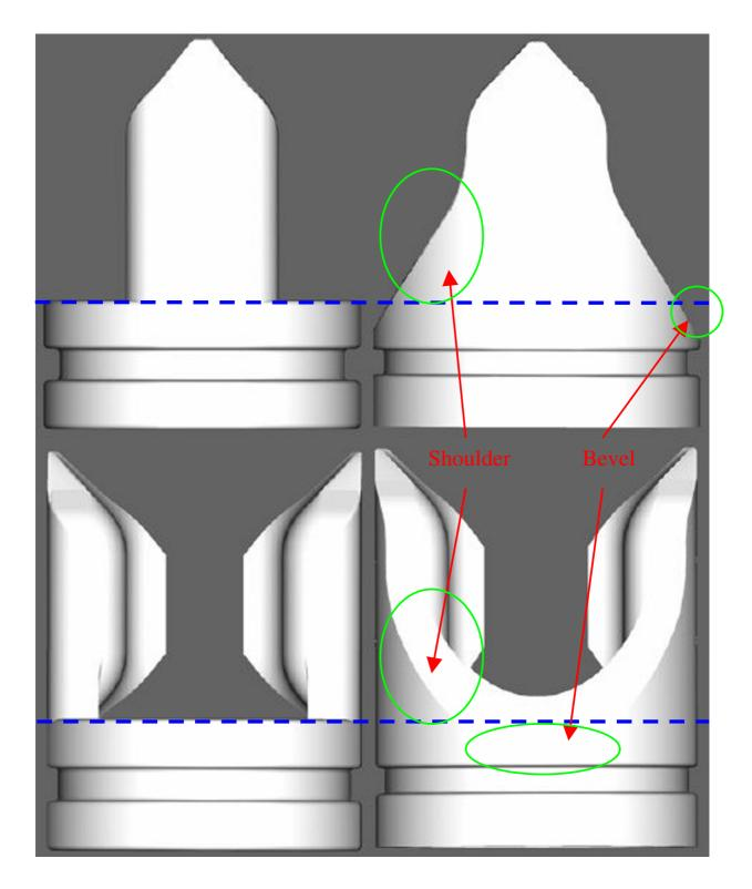
The original (left) and most advanced (right) second-generation frames as depicted in the yz- (top) and xz- (bottom) planes. The additional bevel and shoulder features of the most advanced design are labeled and indicated with arrows.
