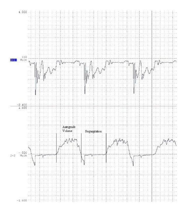
Representative differential pressure (top) and flow rate (bottom) waveforms from the physiologic system under the STBR condition utilizing a second-generation prototypic valve. The division of one cycle associated with the calculation of antegrade and regurgitant volumes is shown.
