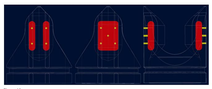
Figure 10 Potential drug delivery reservoir (red) and channel configurations (yellow) as part of the most advanced second-generation design.
