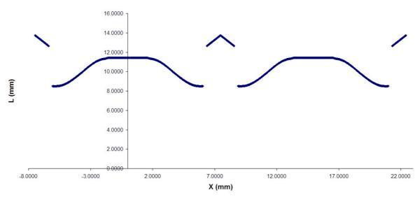
Figure 5 The 2-D leaflet template with L plotted versus X by the spreadsheet program.
