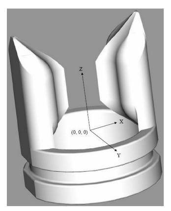
Figure 3 The three-dimensional Cartesian coordinate system utilized for leaflet design.
