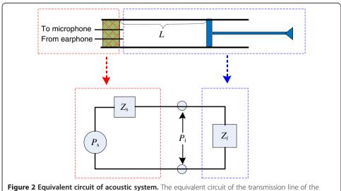
**Figure 2 Equivalent circuit of acoustic system.** The equivalent circuit of the transmission line of the acoustic system.
