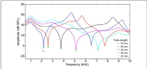
**Figure 5 Sound pressure levels at the tube entrance.** The amplitude spectra of the sound pressure levels at the entrance of the tube  $(P_i)$  as functions of five effective tube length. The asterisks indicate the first notch frequency  $(f_0)$  of  $P_i$ .
