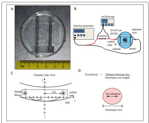
**Figure 1 Chamber Design, Electric Field Setup and Strength Calculations**. (a) Carbon electrode chamber design for capacitively coupled field (b) Electric field setup including function generator for power supply and oscilloscope for electric field strength verification (c) Chamber side view outlining chamber dimensions for field strength calculations (d) Cell dimensions for morphological assessment.
