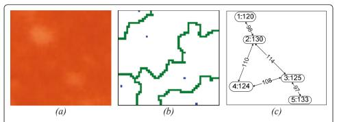
**Figure 7 Merging Algorithm**. This figure shows the segmentation (b) of a small region of a retina image (a) and its corresponding connectivity graph (c). The connectivity graph represents the connections between segmentation areas and is labelled with the minimum intensity border value on each *link*. Each node contains the label and the intensity maximum of the segmentation area it represents.
