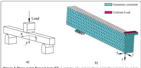
**Figure 3 Three-point flexural test (FT)**. Geometry of a typical three-point flexural test (a) and its corresponding FE mesh with two planes of symmetry (b).
